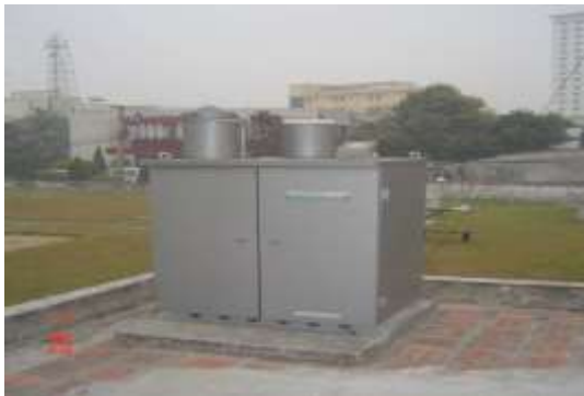
Wet Sampler with pH, EC automatic measurement each mm of rainfall (Kimoto MCSAM-6-VB)
