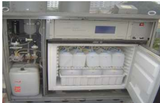
Wet Sampler with pH, EC automatic measurement each mm of rainfall (Kimoto MCSAM-6-VB)
